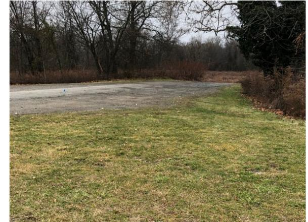
A rain garden can be installed in the turfgrass area to the northwest side of the gravel road to capture, treat, and infiltrate stormwater runoff from the road. Two rain gardens could be installed near the building to capture runoff from the rooftop. A preliminary soil assessment suggests that more soil testing would be required before determining the soil's suitability for green infrastructure.
